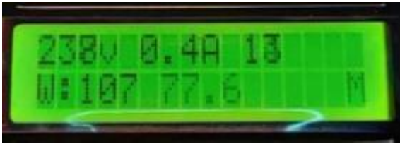
Figure 7. LCD displaying voltage ,current and wattage reading
