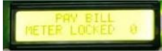
Figure 9. LCD displaying message “Meter locked” when previous month bill is unpaid
