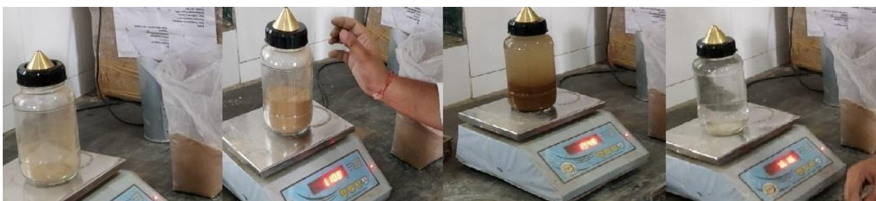
Figure 2 Pycnometer test on desert sand.
