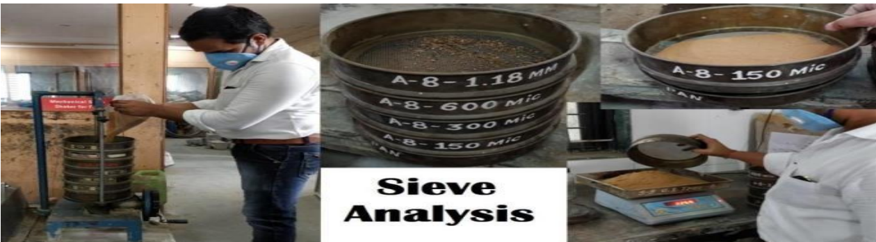
Figure 1 Sieve analyses test on desert sand
